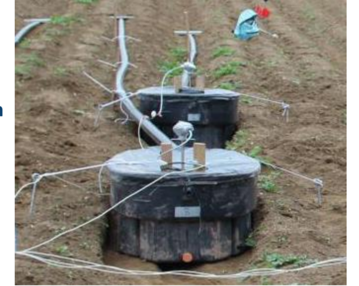
Collection Tank with linear level sensors
